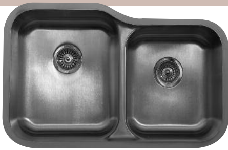
Model: E-260R Outside dimensions: 32 3 / 4 " x 20 7 / 8 " Inside bowl dimensions: Left bowl: 15 1 / 4 " x 18 3 / 8 " x 8" Right bowl: 13 1 / 2 " x 16 1 / 4 " x 7 1 / 4 " Bowl divide height: 6 1 / 8 " Gauge: 18
