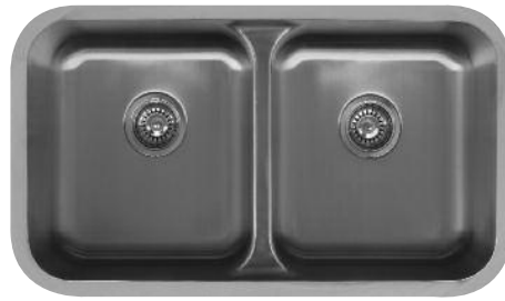
Model: E-250 Outside dimensions: 32 7 / 8 " x 19" Inside bowl dimensions: Left bowl: 14 1 / 2 " x 16 5 / 8 " x 8" Right bowl: 14 1 / 2 " x 16 5 / 8 " x 8" Bowl divide height: 6 1 / 4 " Gauge: 18
