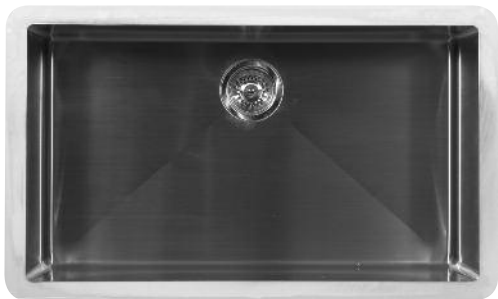
Model: E-540 Outside dimensions: 32 1/2" x 19 1/2" Inside bowl dimensions: 30" x 17" x 9" Gauge: 18
